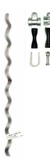
The Preformed Armor-Grip Suspension unit is intended for use on all material types and conductor constructions. Designed to reduce the static and dynamic stresses at the support point so that the conductor is protected against the effects of conductor motion. It also protects the conductor in the support area against impulse and power flash-over arching.
